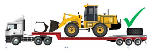
**2.2.4** Multiple items must not be loaded front to back on a rigid truck and pig trailer (or tag trailer) combination if it results in the length, measured from the front of the vehicle combination to the rear of the load, exceeding 20 metres in overall length or an allowable vehicle dimension limit, such 12.5 metres for the rigid vehicle, or 3.7 metres rear overhang.
