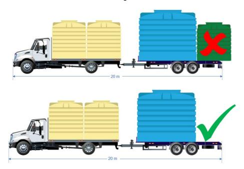
**2.2.5** Multiple items must not be loaded front to back on a rigid truck and dog trailer combination, if it results in the length exceeding 25 metres in overall length or an allowable vehicle dimension limit, such 12.5 metres for the rigid vehicle, or 3.7 metres rear overhang.
